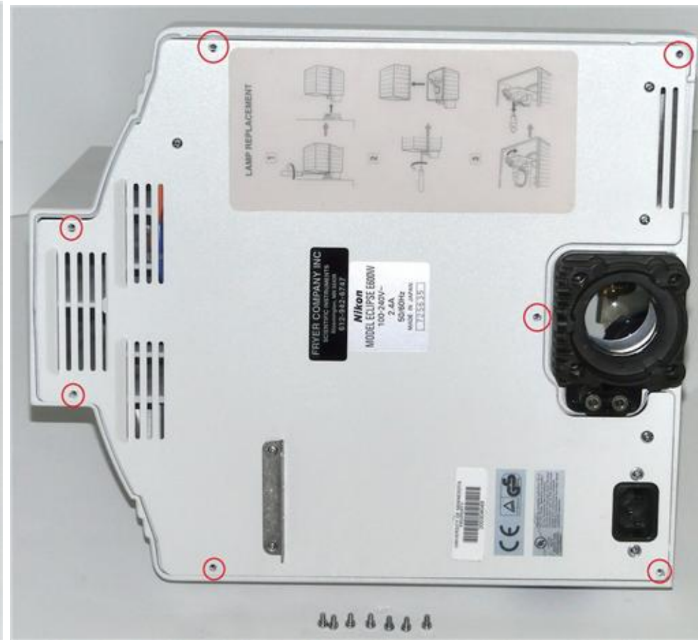
(3): Remove the back cover. It is held by 7 screws (at the red circles in the photo above).
