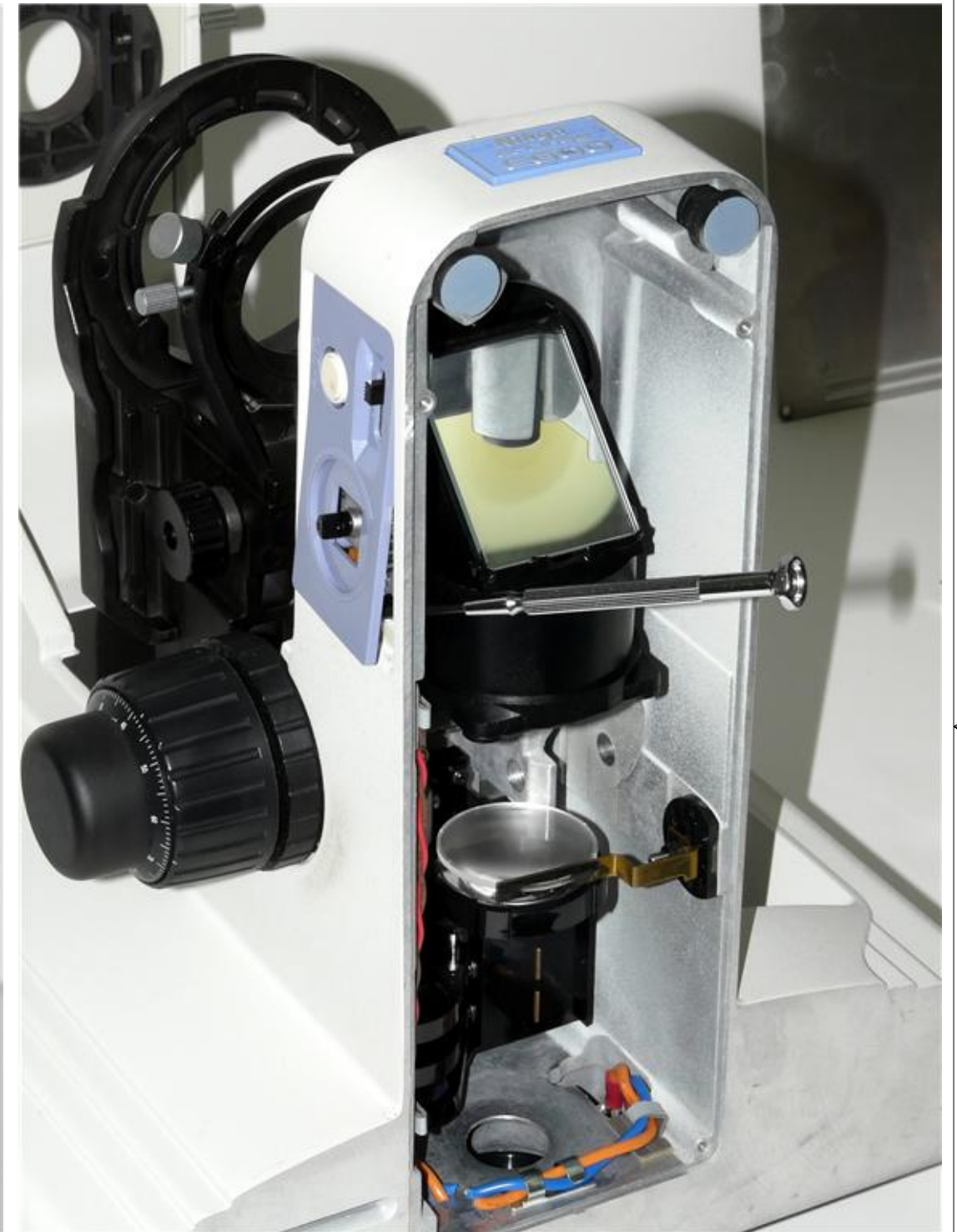
(2): Remove the plastic potentiometer plate as shown above. Push it out from the inside. Use a small screwdriver or similar tool if needed.
