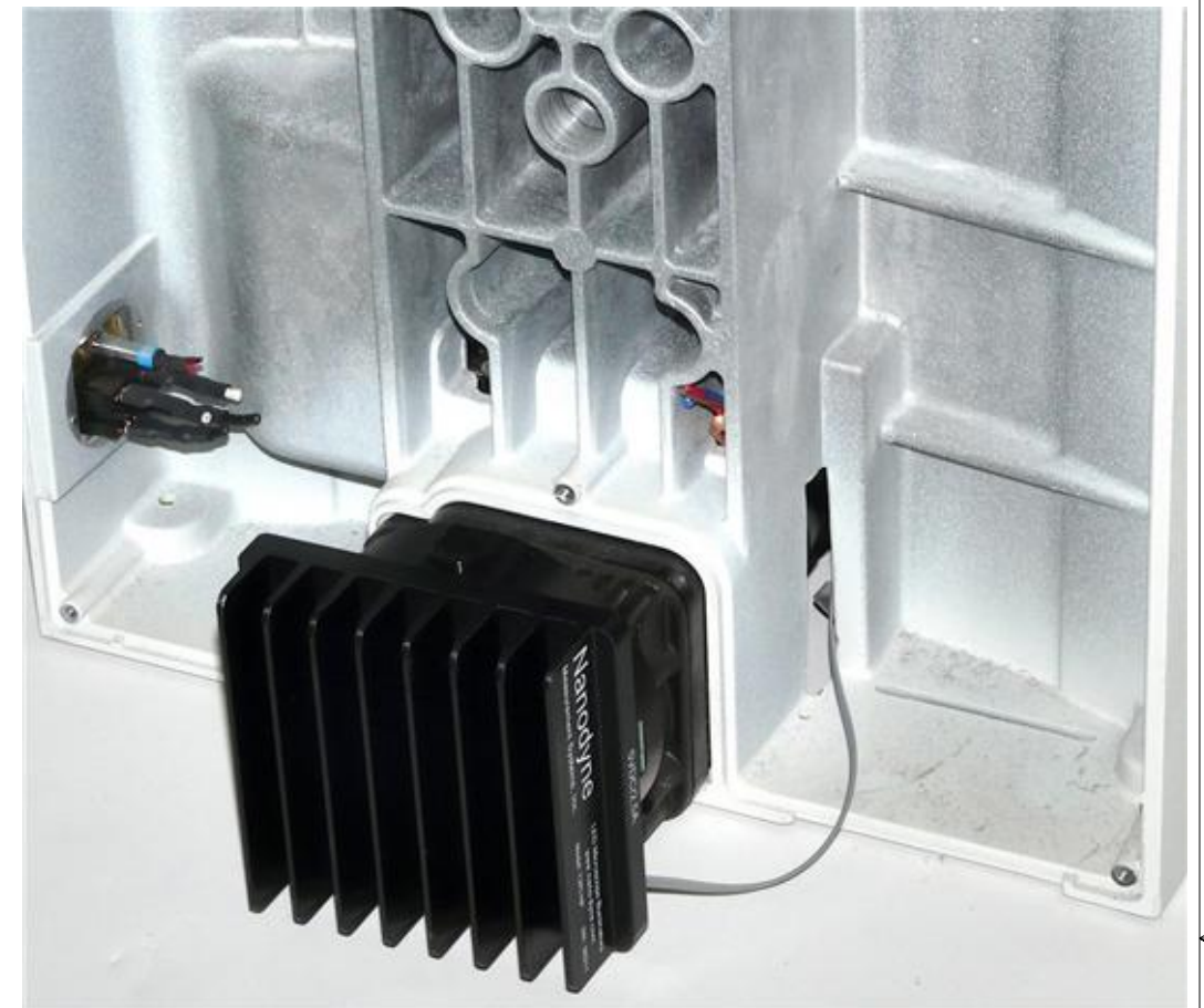
(3): Connect the pot cable to the socket on the bottom of the illuminator.
