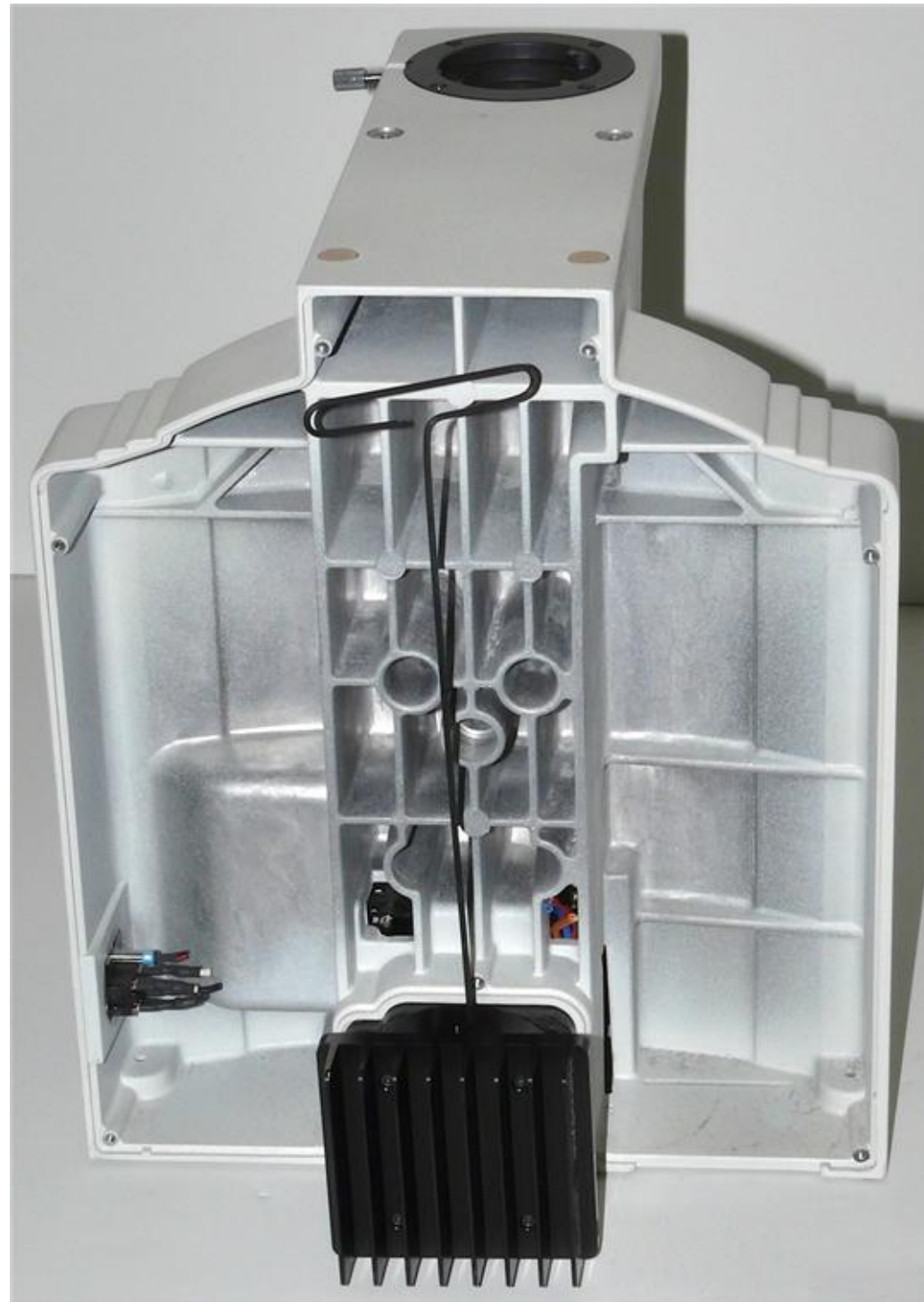
(2): The new illuminator fits just like the old one. Secure it by tightening the set screw with the 2mm hex key provided.
