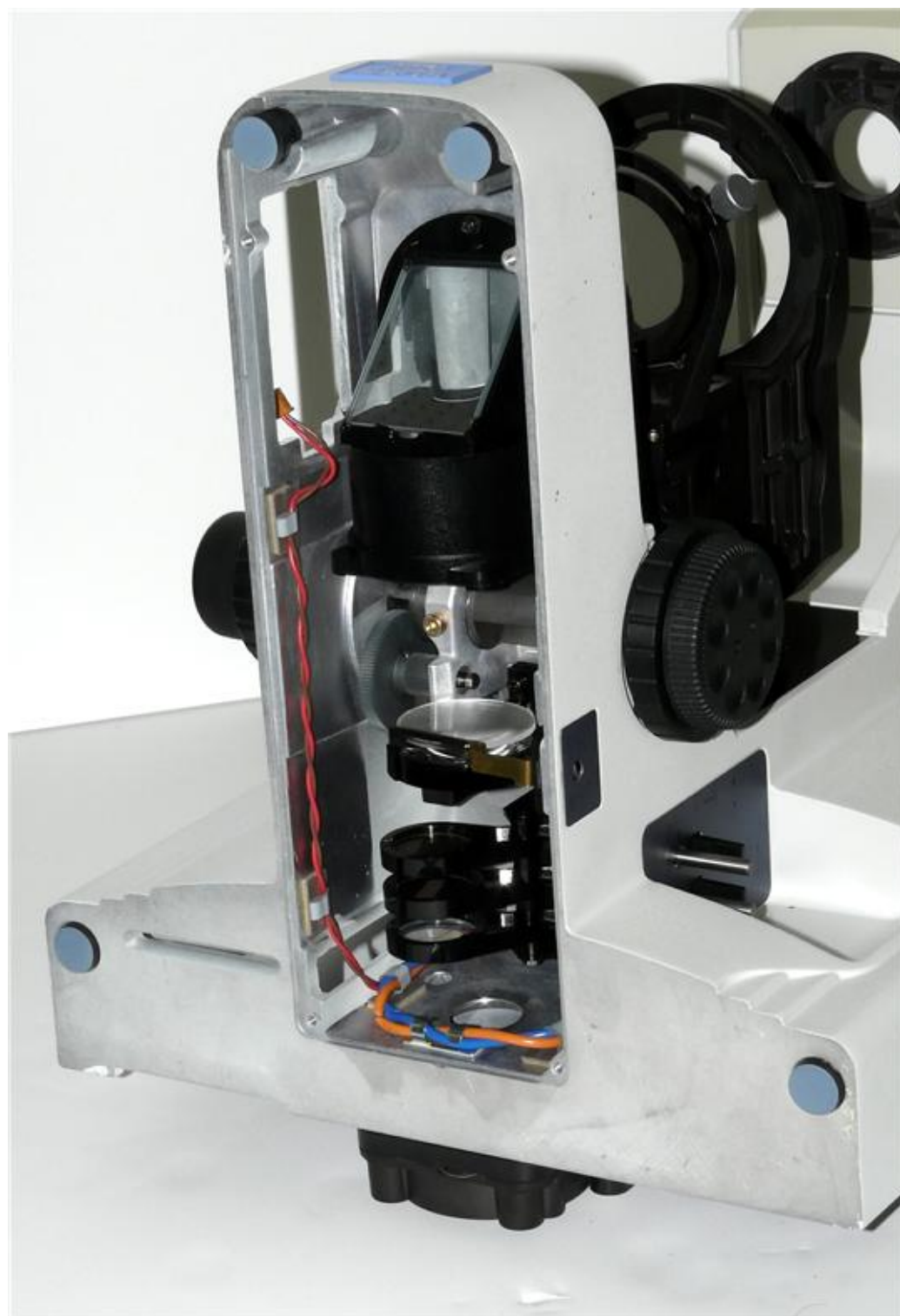
(1): Disconnect and remove the wires that go from the old pot plate to the old power supply.
