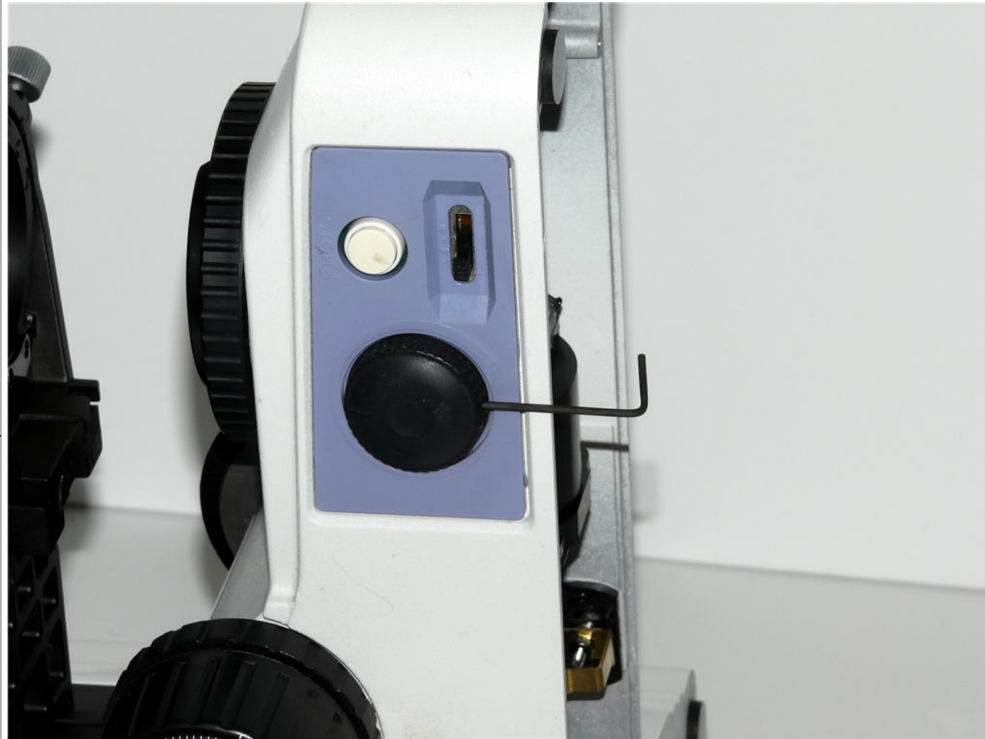
(1): Remove the potentiometer knob from the microscope using the 1.5mm hex key provided. The knob will be re-used for the new illuminator.
